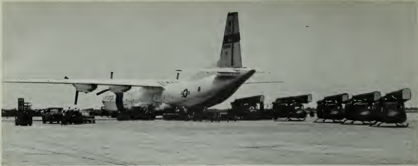
Five For Three—That's story of how five Huey helicopters, instead of three, can be loaded into Cargomaster transports by placing tailbooms atop the choppers.
