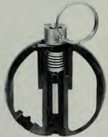
Another, shown in cutaway model, is size of baseball.
