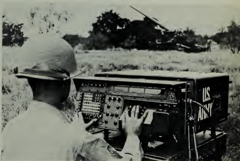
Left, van housing part of computer system is loaded for shipment to Vietnam. Above, Direct Support Unit/General Support Unit System speeds supply procedures through computers. Right, Field Artillery Digital Automatic Computer (FADAC) is used in field firing calculations.
