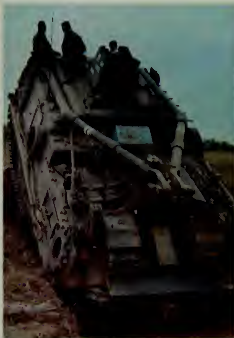
Tank recovery vehicle doubles by digging emplacement for an armored track vehicle.
