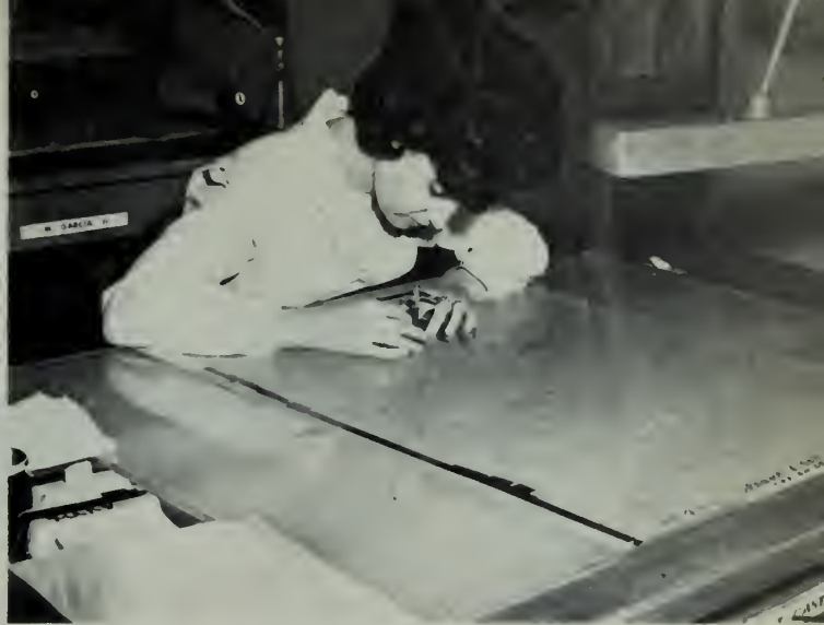
Magnifying glasses, special tools, are required in scribing process in making maps—here coast line is being detailed on special transparency film.
